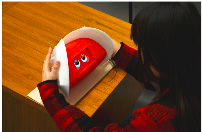
Fig. 2. A social robot prototype combining facial expression and the texture changing skin. During human-robot interaction, the user puts their palms on the shells for haptic feedback and makes eye contact with the screen face.
